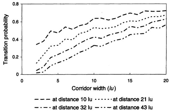
Fig. 5. These curves correspond with the simulations 'DW' combined with 'Turn around' (see Fig. 2e) and show exemplarily that the transition probability increases asymptotically towards an upper level. This asymptotic increase is basically determined by the relationships between P/A and BP (see Fig. 4). The maximum attainable transition probability depends on movement velocity and decreases with increasing distance for a fixed period of time.
